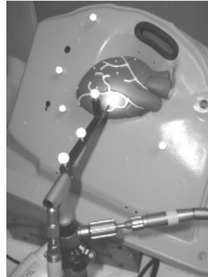
Fig. 1 Optically tracked endoscope pointing at the tracked heart phantom.
