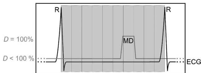
FIG. 1. Data acquisition protocol showing prospective modulation of x-ray tube current (dose D ) between 100% at mid-diastole (MD) and a reduced fraction elsewhere. Following acquisition, the data are binned according to the ECG and reconstructed into one high SNR frame at MD and low SNR frames elsewhere.
