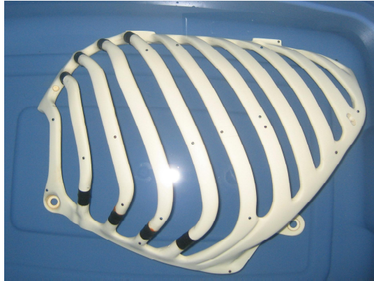
Figure 2. The rib cage phantom. The rib cage phantom was used in all experimentation. Fiducial markers were affixed to the surface of the ribs. For the US acquisition, the rib cage phantom was placed in a 7% (by weight) glycerol-water solution, to mimic the speed of sound of human tissues.
