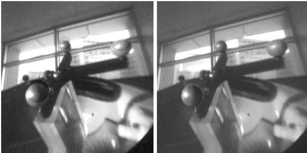
Fig. 2. Proper alignment of the markers in the endoscopic view with their virtual counterparts is achieved through applying the correction transform (right). The corresponding uncorrected image is shown on the left. Each of the three spherical markers visible in the pictures is 11.5 mm in diameter. While the virtual markers are shifted from the locations in the optical locations in the uncorrected image, the shift is reduced in the corrected image.
