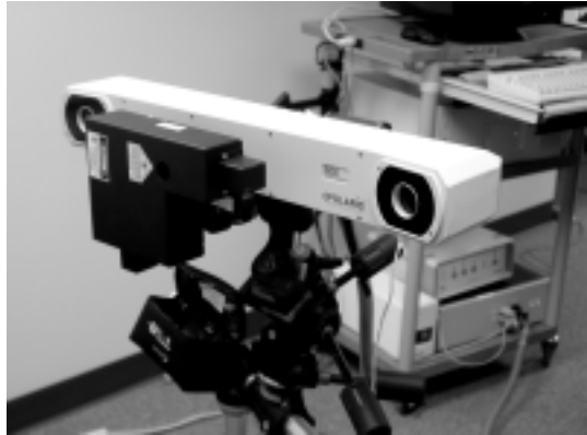
Fig. 1. The XarTrax device mounted upon a POLARIS optical tracking system.
